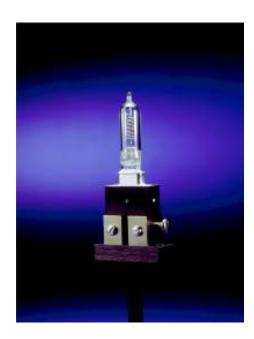
Gooch and Housego offers 1000-W FEL type lamps as standards of spectral irradiance, total irradiance, Illuminance, and color temperature. These lamps have a tungsten coiled-coil filament enclosed in a small quartz envelope. The lamp bases have been converted to a medium bi-post base as recommended by the National Institute of Standards and Technology (NIST). This special lamp base improves alignment accuracy, which minimizes uncertainties due to positioning and orientation of the lamp.
