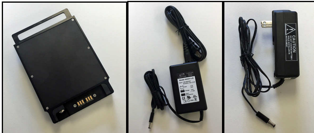
Figure 7 Battery Pack (Left), Fast-Charger (Middle), and Standard Charger (Right)
