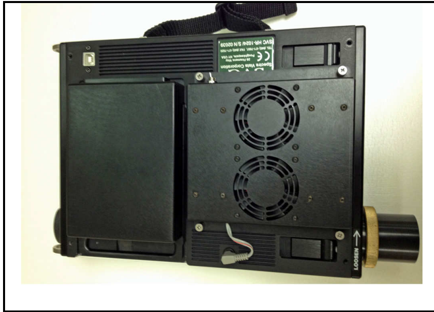
Figure 16 Instrument Optical Plate After Fan Installation
