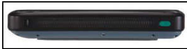
Figure 10 Juno T41 PDA Side View Showing Green Reset Button
