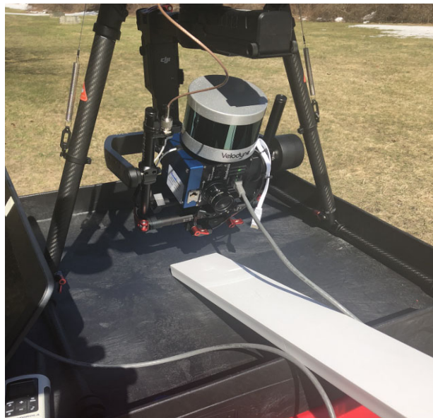
Figure 2-25. Nano Aimed at White Reflectance Target
