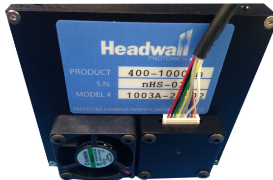
Figure 1-9. Cable Connector secured in Nano Connector Housing.
