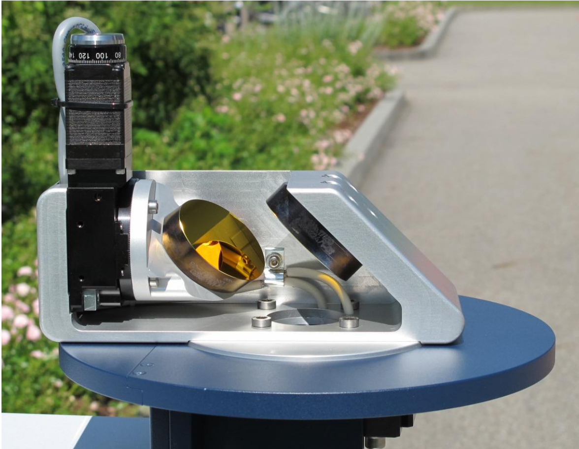
Figure 1: The solar tracker of the EM27/SUN
