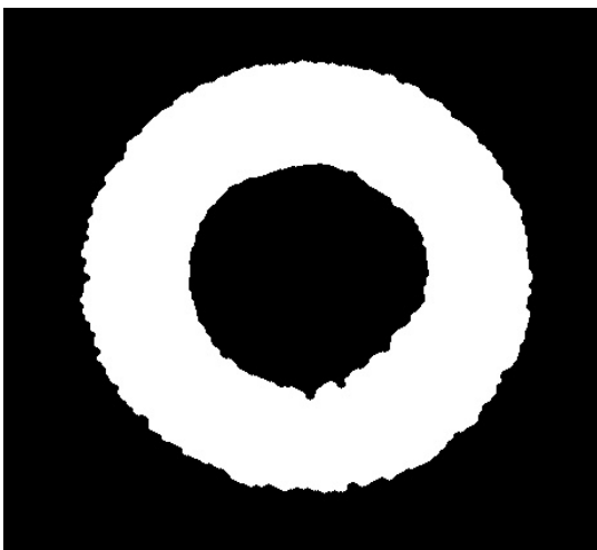
Figure 10: Solar image after conversion to a binary image. The black areas correspond to intensity values below a threshold value.
