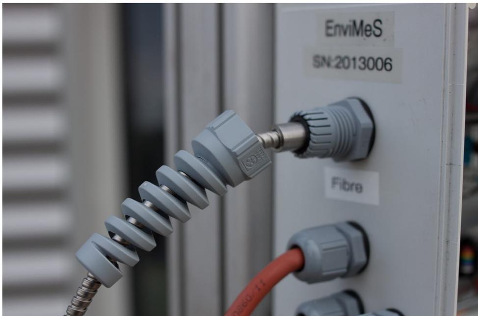
Figure 4: Before tightening the PG plug, the fibre, the stainless steel tube and the rubber sealing should look like this.
