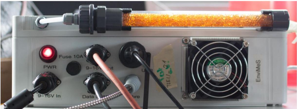
Figure 2.2: The front of the spectrometer box. From left to right: Power switch, power connector, 10A fast fuse, 9-16V power supply telescope scanner unit, data cable for scanner, airtight USB connector to computer, fibre, heatsink. On top is a tube of desiccant, which should be changed when the color has changed from orange to green and blue entirely.
