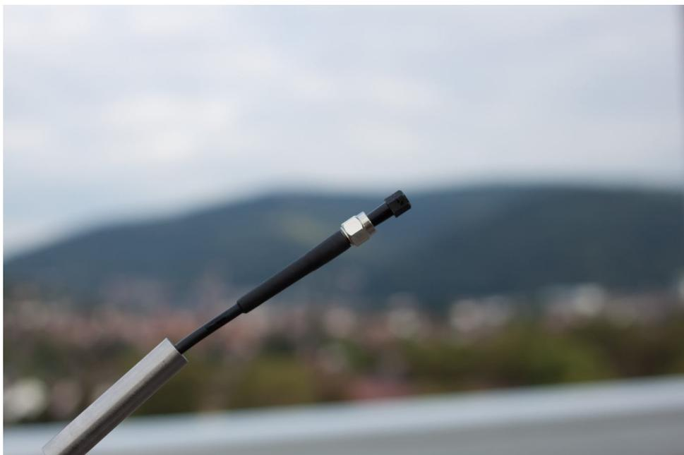
Figure 2: The end of the fibre, protected by a black cap. On the left the stainless steel tube can be seen which is used to close the scanner unit.
