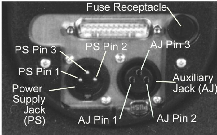
Please refer to the 'Set-up Section' of this manual for instructions on the proper installation of the Power Supply. The Switchcraft Connector Power Supply Jack, Auxiliary Jack and Power Fuse are located on the lower backside of FieldSpec® Pro, details above.
