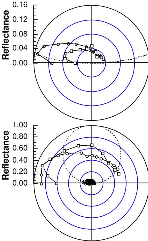
Figure 6. Bi-directional reflectance functions (BRDF) of a conifer, Mugo Pine, (circles) and a broadleaf shrub, Viburnum, (squares). For reference, the BRDF of a lambertian reflector is plotted as a dashed line. The left plot is for a red band (650 nm) and the right plot is for a near infrared band (850 nm). Both canopies were illuminated from the left at an elevation of about 30°.
