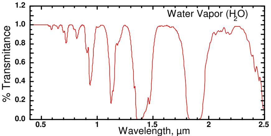
Figure 3. Transmission spectrum of water vapor for typical atmospheric conditions.
