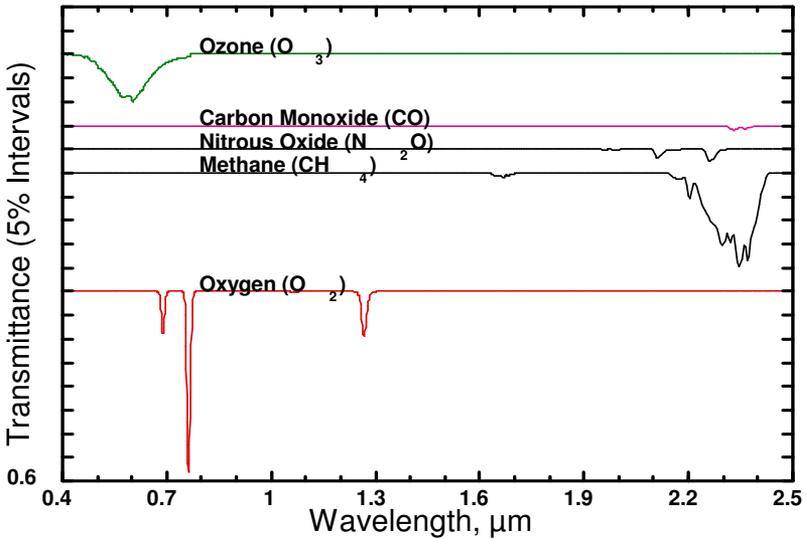
Figure 5. Transmission spectrum of various gases for a typical atmospheric conditions.
