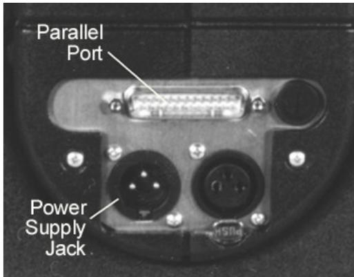
Making sure that the Switchcraft Plug holes align with the Jack pins and that the release clip is pointing downward, push the
