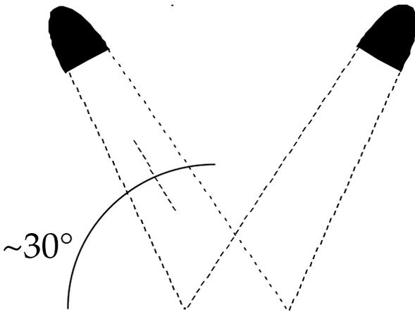
Figure 2. A typical lamp configuration for artificial illumination; the sample is viewed with the collecting optics of the spectrometer nadir to the sample. Use 1 or 2 200 to 500 Watt quartz-halogen cycle tungsten filament lamps (~3400°K color temperature) in housings with aluminum reflectors about 1 meter above the surface being measured.
