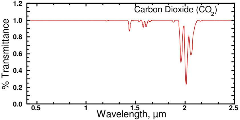
Figure 4. Transmission spectrum of carbon dioxide for typical atmospheric conditions.
