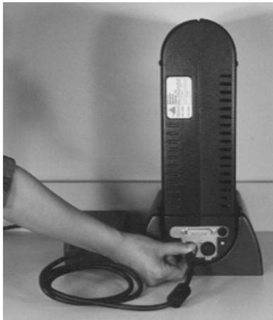
Switchcraft Plug into the left Jack as shown in the picture on the below. You should hear a click and then the Switchcraft Plug should be firmly connected.
