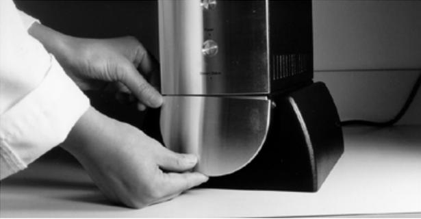
Pull/pop out the bottom of the front bezel plate as shown in the picture above, note the FieldSpec® Pro's plate is plastic.
