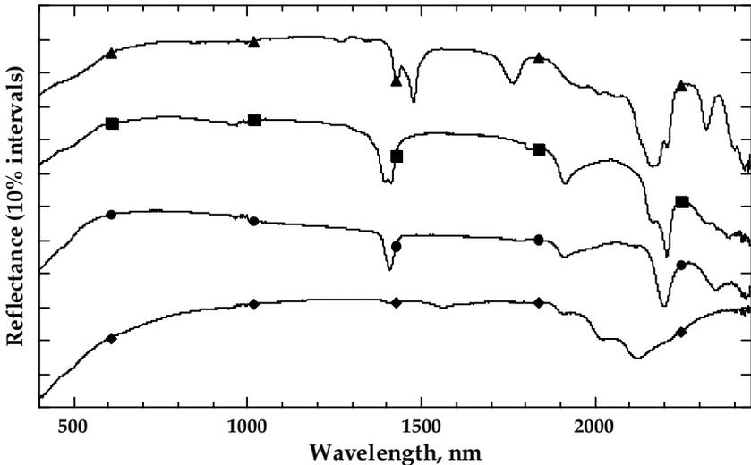
Figure 7. Reflectance spectra of alunite (triangles), kaolinite (squares), illite (circles), and buddingtonite (diamonds) measured with a FieldSpec® FR field portable spectroradiometer.
