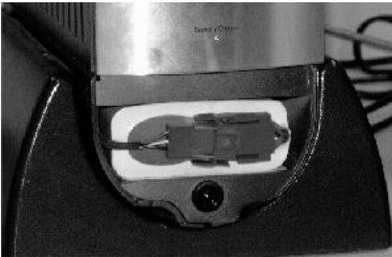
To remove the battery, press on the Cable Connector clips and gentle pull the two halves from one another as shown below.
