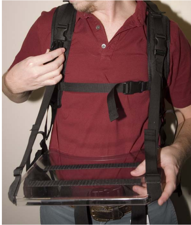
Figure 13-8 ASD spectroradiometer (such as the FieldSpec3) in the Ergonomic Pro-Pack and instrument controller on the belly board.
