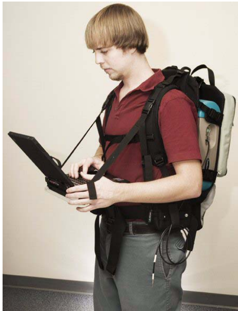
Figure 13-8 ASD spectroradiometer (such as the FieldSpec3) in the Ergonomic Pro-Pack and instrument controller on the belly board.
