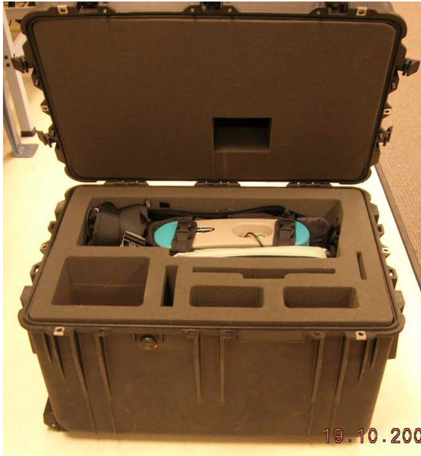
Figure 13-1 Shipping case with Ergonomic Pro-Pack with ASD spectroradiometer (such as the FieldSpec3) and instrument controller.
