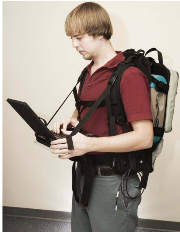
Figure 6-16 FieldSpec spectroradiometer in the Ergonomic Pro-Pack and instrument controller on the belly board.
