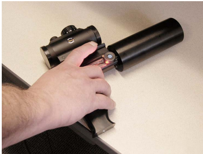
Figure 2-14 Pistol grip with red-dot scope (sold separately), one degree field of view (sold separately), and trigger (standard) attached.
