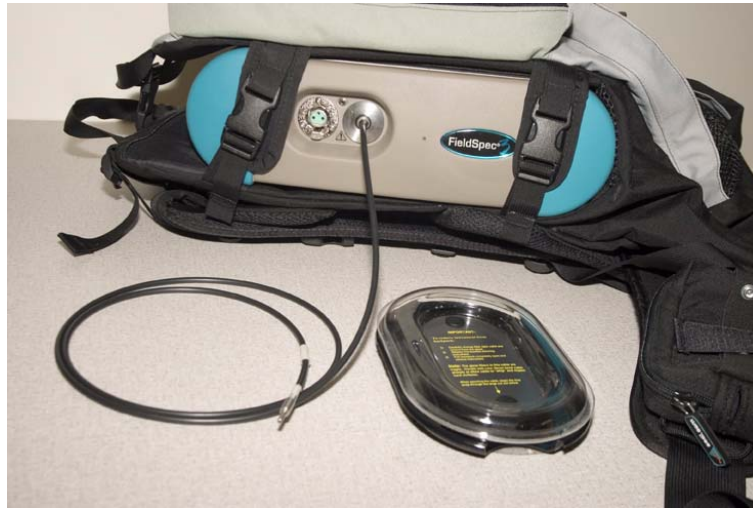
Figure 6-8 Fiber optic cable routes to either side.
