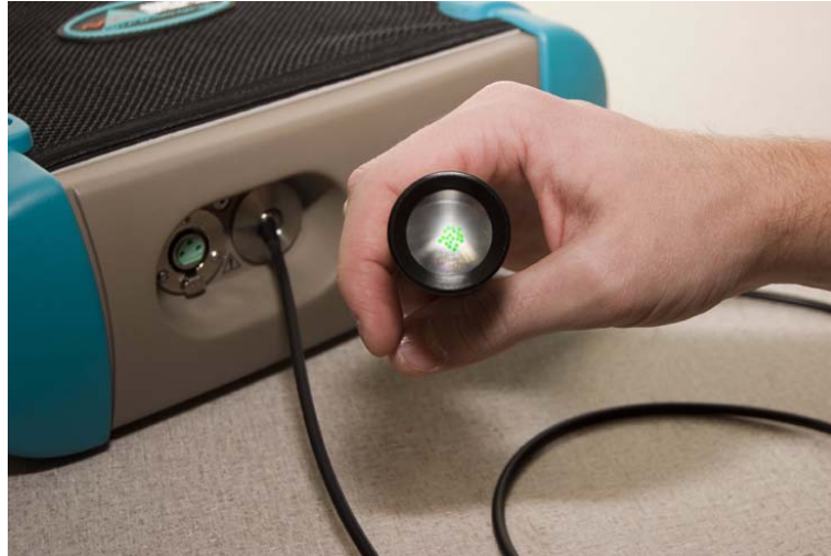
Figure 4-3 Internal spectrometer LED shining to test fiber optic cable.
