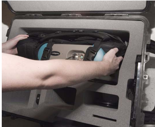
Figure 6-6 Placing the Ergonomic Pro-Pack with FieldSpec spectroradiometer and instrument controller into the shipping case.
