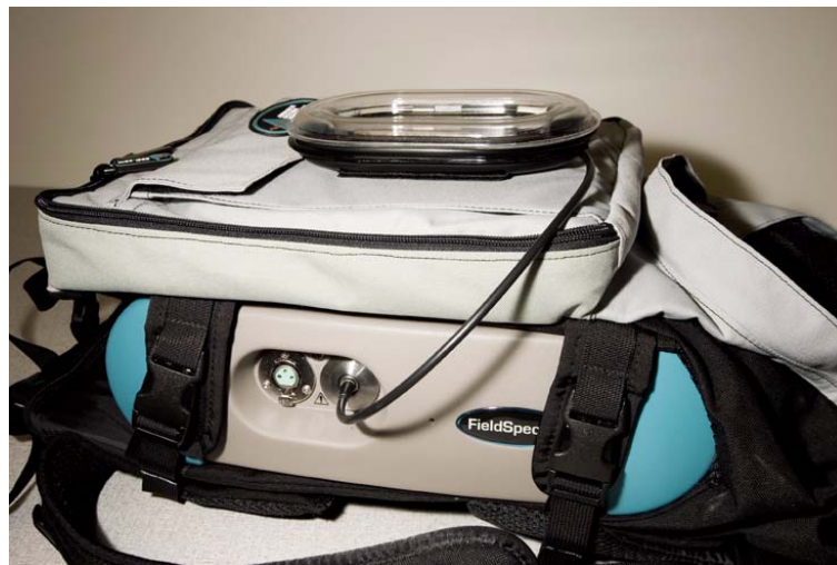
Figure 6-9 Fiber optic spool on the outside of the Ergonomic Pro-Pack (with velcro).
