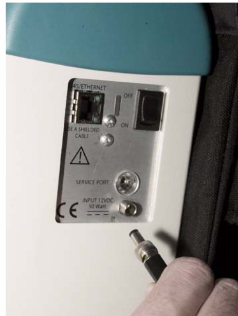
Figure 2-10 FieldSpec spectroradiometer back panel showing Ethernet connection, power switch, and power input jack.
