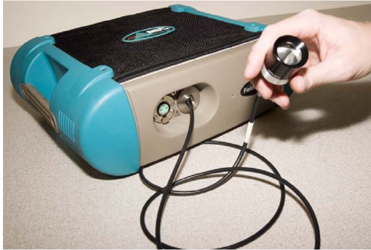
Figure 4-1 Magnifier for testing the fiber optic cable.
