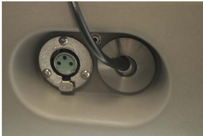
Figure 2-12 Enhanced view of the front panel with the fiber cable connector and accessory power port.
