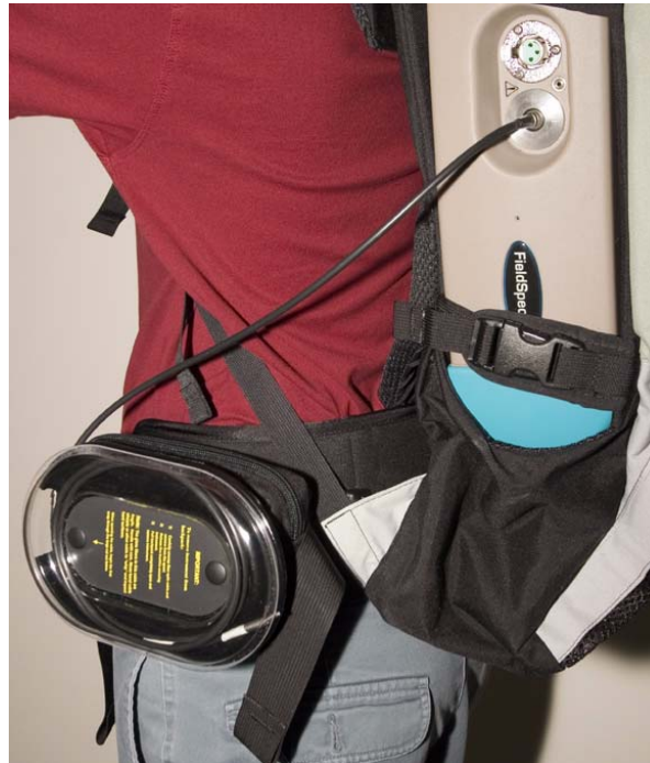
Figure 6-14 Fiber optic cable spool on the battery pouch on the hip belt.
