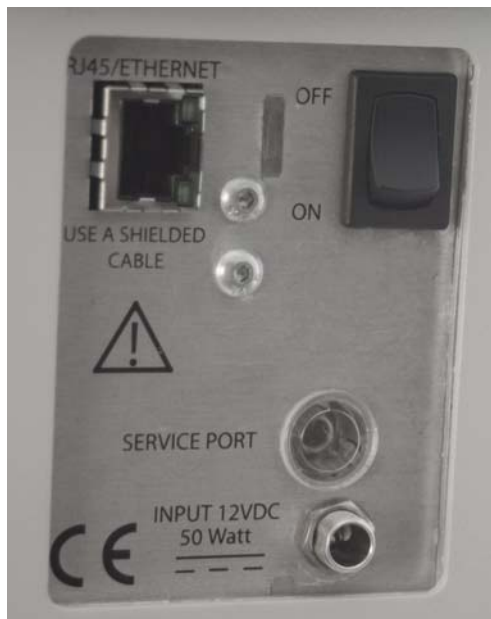
Figure 2-10 FieldSpec spectroradiometer back panel showing Ethernet connection, power switch, and power input jack.
