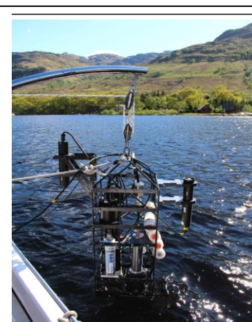
Fig 1. The FSF optics suite being used to measure the optical properties on Loch
