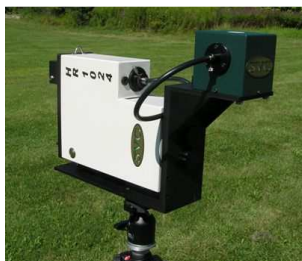
The Facility's new SVC HR-1024 full wavelength system, here with integrating sphere fitted.
