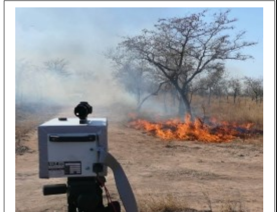
FTIR in open path mode measuring fire emissions
